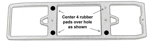
Install 4 self-adhesive rubber pads on the inside of each side panel
